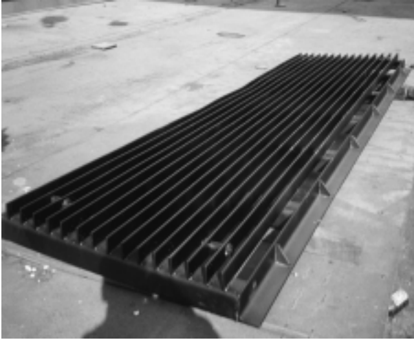
圖 9. 興達火力發電廠試驗架。 Figure 9. The test frame Power Plant is ready for immersion in Shin-Der Power Plant.
